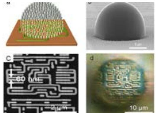
(a) Conceptual drawing of nanoparticle-based metamaterial solid immersion lens (mSIL) (b) Lab made mSIL using titanium dioxide nanoparticles (c) SEM image of 60 nm sized imaging sample (d) corresponding superlens imaging of the 60 nm samples by the developed mSIL. Credit: Bangor University Fudan University
