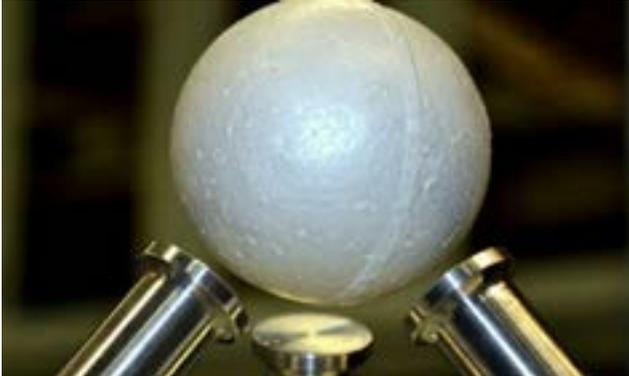
Acoustic levitation of a polystyrene sphere, the first spherical object to be acoustically levitated that is larger than the acoustic wavelength. Credit: Andrade et al. ©2016 AIP Publishing
