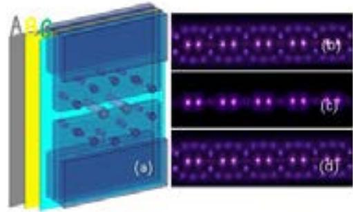
A schematic diagram of the spatial distributions of the pattern in three cross sections A, B and C along z axis. (a) A sketch of three dimensional pattern. (b-d) Schematic diagram of the spatial distributions of the pattern in cross section A, B and C denoted in (a). Credit: Hebei University
