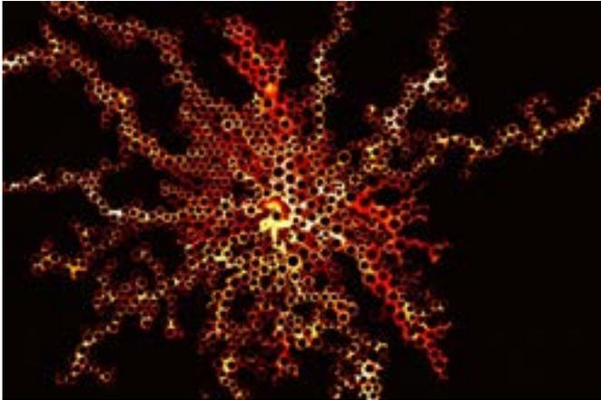
Lab simulations carried out by an MIT and Oxford University team provide detailed information about how a liquid moves through spaces in a porous material, revealing the key role of a characteristic called wettability. Credit: Massachusetts Institute of Technology
