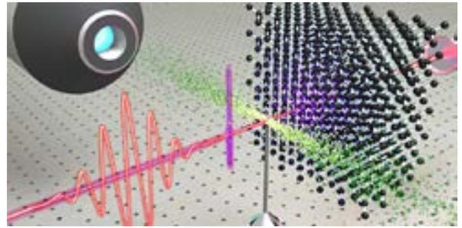
A short laser pulse travels through a diamond (black spheres) and excites electrons inside it. The strength of the excitation is measured using an attosecond ultraviolet pulse (violet). Credit: Matteo Lucchini, ETH Zurich
