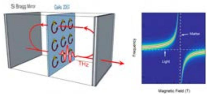
A method created at Rice University closes the gap between light and matter and may help advance technologies like quantum computers and communications. The lab designed and built a high-quality cavity to contain an ultrathin layer of gallium arsenide. By tuning the material with a magnetic field to resonate with a certain state of light in the cavity, they prompted the formation of polaritons that act in a collective manner. Credit: Qi Zhang/Rice University
