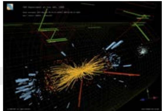
Real CMS proton-proton collisions events in which 2 high energy electrons and two high energy muons are observed. Credit: Taylor L; McCauley T/CERN
