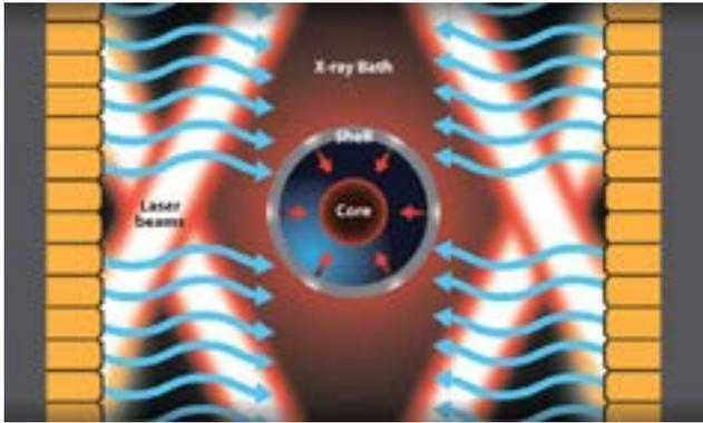
In the indirect-drive method of inertial confinement fusion, laser beams are converted to x-rays. Credit: Michael Osadwic/University of Rochester.
