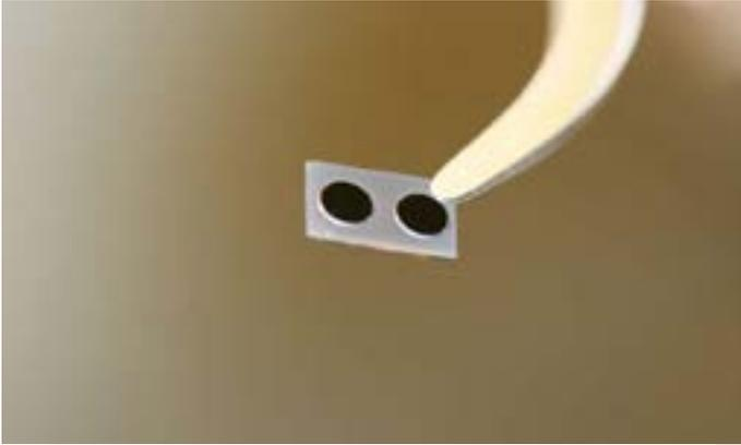
Optical microcavities in which the solitons were created. Credit: Qi-Fan Yang/Caltech
