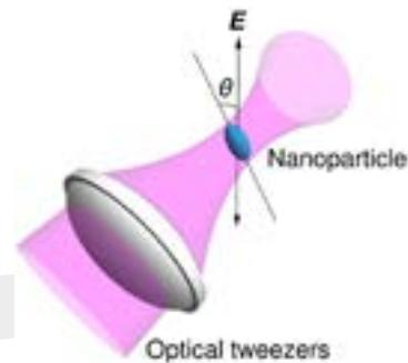
This graphic represents a new experiment where levitating a nanodiamond with a laser in a vacuum chamber for the first time was used to detect and measure its “torsional vibration,” an advance that could bring new types of sensors and studies in quantum mechanics. Credit: Purdue University image/ Thai M. Hoang
