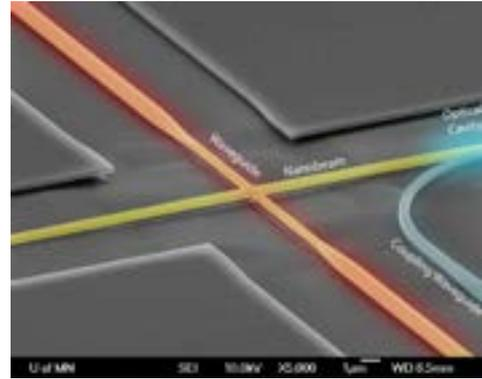
Measurement of the twisting force, or torque, generated by light on a silicon chip holds promise for applications such as miniaturized gyroscopes and sensors to measure magnetic field, which can have significant industrial and consumer impact. Credit: University of Minnesota
