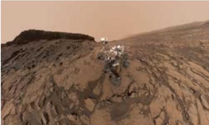
This September 2016 self-portrait of NASA's Curiosity Mars rover shows the vehicle at the "Quela" drilling location in the scenic "Murray Buttes" area on lower Mount Sharp. The panorama was stitched together from multiple images taken by the MAHLI camera at the end of the rover's arm. Image courtesy NASA/JPL-Caltech/MSSS.
