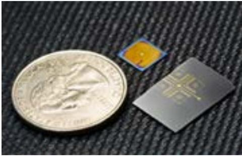
An optically-driven mechanical oscillator fabricated using a plas-momechanical metamaterial. Credit: UC San Diego Jacobs School of Engineering
