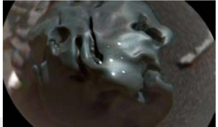
The dark, golf-ball-size object in this composite, colored view from the ChemCam instrument on NASA's Curiosity Mars rover is a nickel-iron meteorite, as confirmed by analysis using laser pulses from ChemCam on Oct. 30, 2016. The grid of bright spots on the rock resulted from the laser pulses. Credit: NASA/JPL-Caltech/LANL/CNES/IRAP/LPGNantes/CNRS/IAS/MSSS
