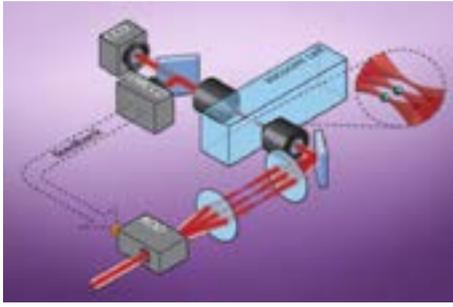
This image shows the basic setup that enables researchers to use lasers as optical “tweezers” to pick individual atoms out from a cloud and hold them in place. The atoms are imaged onto a camera, and the traps are generated by a laser that is split into many different focused laser beams. This allows a single atom to be trapped at each focus. Credit: Massachusetts Institute of Technology
