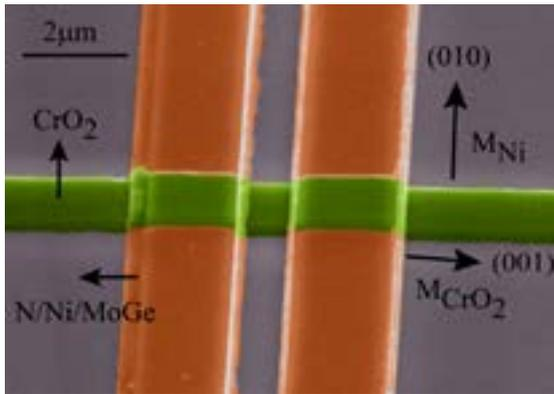
Electron microscope image of a chromium dioxide devices based on wires. The green wire is the chromium dioxide ferromagnet. The orange wires are superconductors and are necessary to produce a superconducting current through the green wire. Credit: Leiden Institute of Physics
