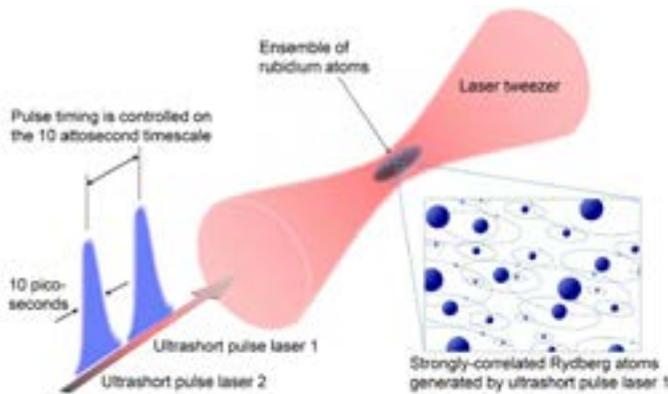
Schematic explanation of the world's fastest quantum simulator. Credit: NINS/IMS
