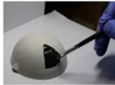
Thermoelectric paint being applied to an alumina hemisphere. The paint provides closer contact with the heat-emitting surface than conventional planar thermoelectric devices do. Credit: Park et al. ©2016 Nature Communications
