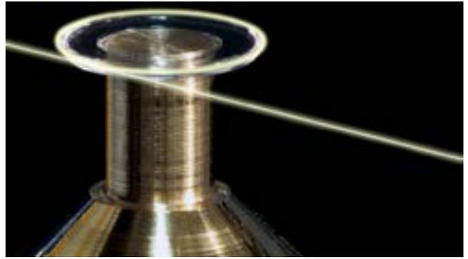
A microresonator crystal used in this study . Credit: © T.J. Kippenberg/EPFL
