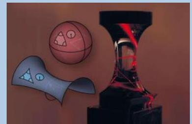
*A laser beam in an experiment propagates along the two-dimensional surface of a glass object shaped like an hourglass, curling once around the middle of the object. This is an example of an object with negative surface curvature (like a saddle, for example), in contrast to an object with positive surface curvature, such as a sphere. Credit: Vincent Schultzeif*
