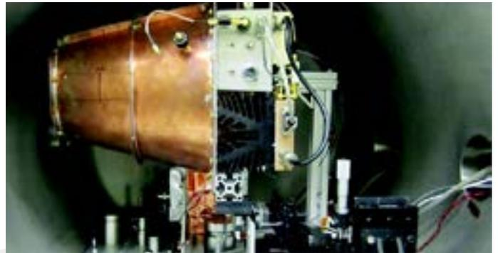
EM Drive in forward thrust configuration. Credit: NASA Photo
