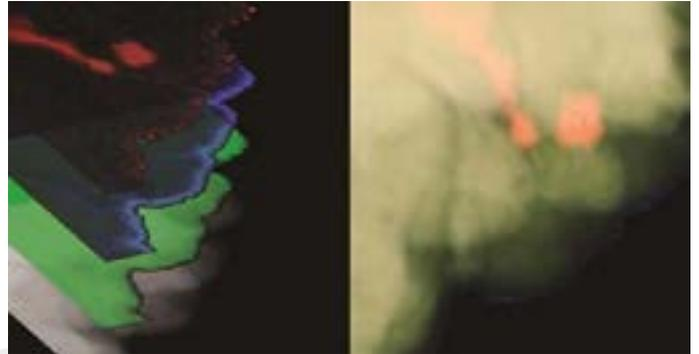
Scanning transmission electron microscope image of a nickel-platinum composite material created at The Ohio State University. At left, the image is overlaid with false-color maps of elements in the material, including platinum (red), nickel (green) and oxygen (blue). Credit: Imaging by Isabel Boona, OSU Center for Electron Microscopy and Analysis; Left image prepared by Renee Ripley. Courtesy of The Ohio State University.
