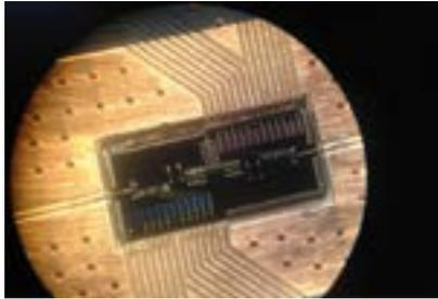
A Princeton University-led team has built a device that advances silicon-based quantum computers, which when built will be able to solve problems beyond the capabilities of everyday computers. The device isolates an electron so that can pass its quantum information to a photon, which can then act as a messenger to carry the information to other electrons to form the circuits of the computer. Credit: Princeton University
