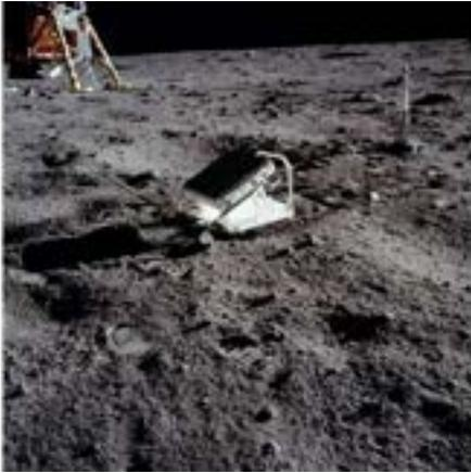
This retroreflector was left on the Moon by astronauts on the Apollo 11 mission in 1969. Astronomers all over the world have reflected laser light off the reflector to precisely measure the Earth-Moon distance. Credit: NASA - NASA Apollo Archive, Public Domain
