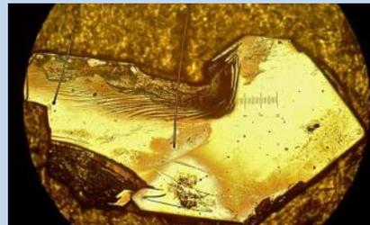
*This microscopic closeup shows a small sample of ytterbium dirhodium disilicide, one of the most-studied 'heavy fermion' composites. The scale bar in the center of the screen is one millimeter wide. Credit: Marc Toppmann/Technical University of Munich*
