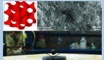
The Wiesner Group at Cornell University has synthesized the first block copolymer self-assembly-derived nanostructured superconductor. Shown is an example of a bismuth-based superconductor levitating a magnet, with simulated and electron microscope images of the nanostructured material. Credit: Cornell University
