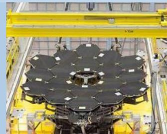
In this rare view, the James Webb Space Telescope's 18 mirrors are seen fully installed on the James Webb Space Telescope structure at NASA's Goddard Space Flight Center in Greenbelt, Maryland. Image courtesy NASA/Cbris Gunn.
