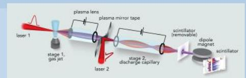
Schematic of the first experiment to achieve staging of laser plasma accelerators (LPAs) with independent laser pulses: a pulse from laser 1 (at left) creates a plasma wakefield in the stage 1 LPA, a gas jet. The resulting electron beam is focused by a capillary-discharge plasma lens and then penetrates a moving tape. Almost simultaneously, an incoming pulse from laser 2 strikes the tape and creates a plasma mirror, which combines the laser beam and electron beam. ....
