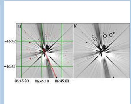
The CID device has the ability to detect dim objects even behind Sirius, the brightest star in our galaxy. The "a" image shows the Sirius field and the sky coordinates in green. Red dots represent already cataloged objects. The red line is the motion of Sirius. The "b" image shows faint objects detected near Sirius.
