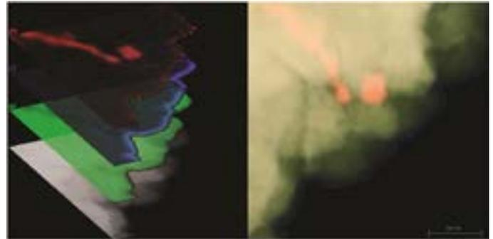
This is a scanning transmission electron microscope image of a nickel-platinum composite material created at The Ohio State University. At left, the image is overlaid with false-color maps of elements in the material, including platinum (red), nickel (green) and oxygen (blue). Image courtesy Isabel Boona, OSU Center for Electron Microscopy and Analysis; Left image prepared by Renee Ripley. Courtesy of The Ohio State University.
