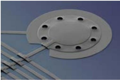
NIST researchers applied a special form of microwave light to cool a microscopic aluminum drum to an energy level below the generally accepted limit, to just one fifth of a single quantum of energy. The drum, which is 20 micrometers in diameter and 100 nanometers thick, beat 10 million times per second while its range of motion fell to nearly zero. Credit: Teufel/NIST
