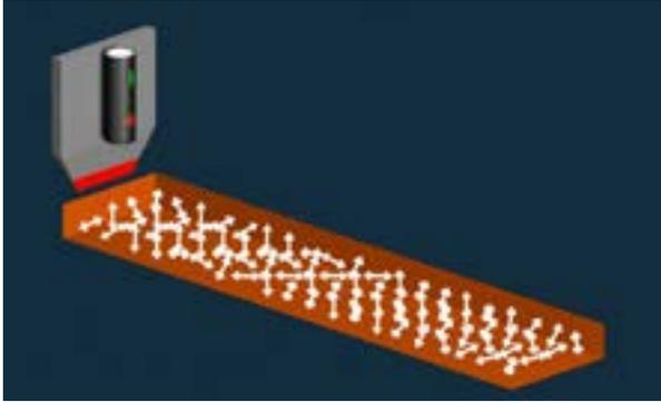
In the experiment, the scientists moved the electric tip along the surface and applied a positive voltage. The electric field aligns the spins of the electrons in the nonmagnetic material, and the ordering creates magnetic properties. If the voltage is reversed, the spins once again become disordered and magnetism is lost. The researchers were able to see the changes using X-ray microscopy at the Stanford Synchrotron Radiation Lightsource. Credit: SLAC National Accelerator Laboratory
