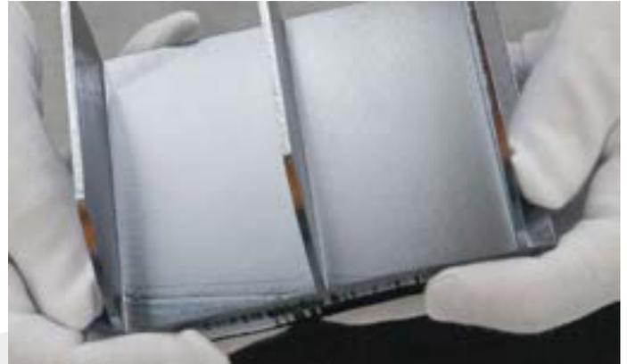
Triple Laue (LLL) neutron interferometer. Credit: Vienna University of Technology
