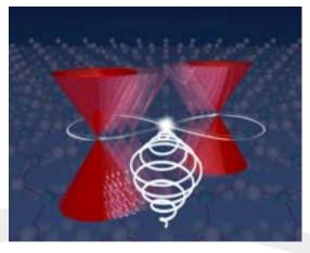
Dancing Weyl cones: When excited by tailored laser pulses (white spiral), the cones in a Dirac fermion material dance on a path (8-shape) that can be controlled by the laser light. This turns a Dirac material into a Weyl material, changing the nature of the quasiparticles in it. One of the cones hosts right-handed Weyl fermions; the other cone hosts left-handed ones. Credit: Joerg M. Harms/MPSD
