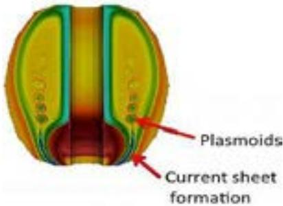
Current sheets and plasmoids are formed during the simulation of a process called coaxial helicity injection, which could produce effective startup current-drive in spherical tokamaks. Image courtesy Fatima Ebrahimi.
