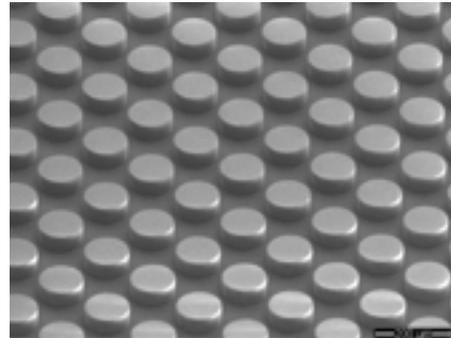
Each cylinder of this new non-metal metamaterial is made of boron-doped silicon and precisely tailored to absorb electromagnetic waves. Credit: Willie Padilla, Duke University
