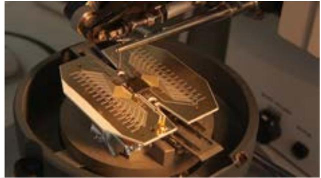
Prototype of the core of a trapped ion quantum computer. Credit: Ion Quantum Technology Group, University of Sussex
