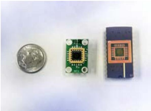
Two different Microelectromechanical devices containing micro mirrors used to position an infrared laser beam to target a receiver and send information. Credit: Patrick Mansell, Penn State
