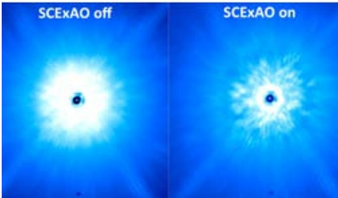
Comparison of images taken from existing, facility instrument (AO 188 + HiCIAO, left) and the newly commissioned instrument (AO 188 + SCExAO, right). Image courtesy NAOJ.
