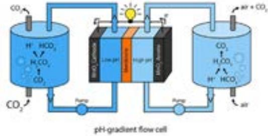
The pH-gradient flow cell has two channels: one containing an aqueous solution sparged with carbon dioxide (low pH) and the other containing an aqueous solution sparged with ambient air (high pH). The pH gradient causes ions to flow across the membrane, creating a voltage difference between the two electrodes and causing electrons to flow along a wire connecting the electrodes. Credit: Kim et al. ©2017 American Chemical Society
