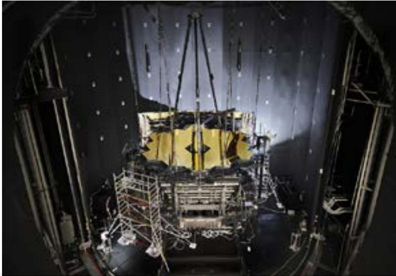
The James Webb Space Telescope is a collaborative project backed by NASA, the European Space Agency, and the Canadian Space Agency. In November 2017, the telescope completed cryogenic testing in Houston; it is now in California with the spacecraft's flight components.
