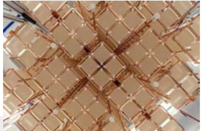
Bottom view of the 19 CUORE towers installed in the cryostat. Credit: CUORE Collaboration
