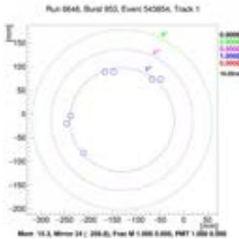
CERNNA62's candidate event of a rare kaon decay. Octagons show hits in the RICH detector. Circles show predicted "Cherenkov rings" for positively charged pion (+), positively charged muon (+) and antielectron ( $e^-$ ) decay particles. Credit: NA62/CERN
