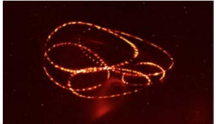
Five superimposed images of W7-X magnetic surfaces displaced by changes in application of trim coil currents. Credit: Max Planck Institute of Plasma Physics
