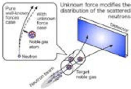
Principle of the experimental test of the inverse-square law of the gravity in nano-meter scale via neutron scattering. Deviation from the inverse-square law will be observed as the modification in the angular distribution of the scattered neutrons.
