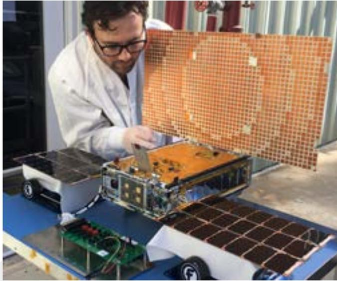
Engineer Joel Steinkraus uses sunlight to test the solar arrays on one of the Mars Cube One (MarCO) spacecraft at NASA's Jet Propulsion Laboratory. Credit: Jet Propulsion Laboratory
