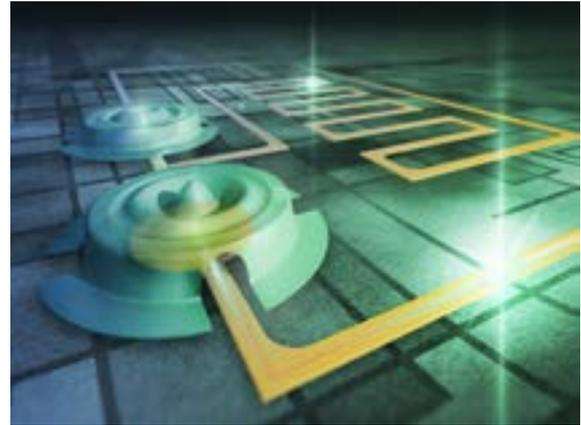
[Illustration of the 15-micrometre-wide drumheads prepared on silicon chips used in the experiment. The drumheads vibrate at a high ultrasound frequency, and the peculiar quantum state predicted by Einstein was created from the vibrations. Credit: Aalto University/Petja Hyttinen & Olli Hanhiova, ARKH Architects.](#)
