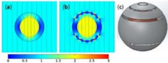
Simulation of a spherical shell that cancels the distortions caused by a ferromagnetic sphere, making the sphere invisible (magnetically undetectable) from the outside. Credit: Mach-Batlle et al. ©2018 American Institute of Physics
