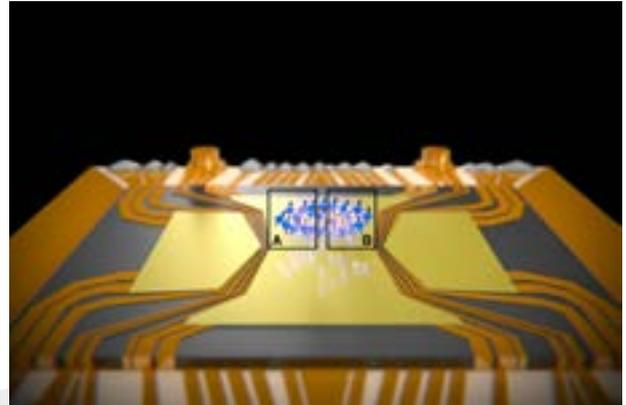
A cloud of atoms is held above a chip by electromagnetic fields. The EPR paradox was observed between the spatially separated regions A and B. Credit: University of Basel, Department of Physics
