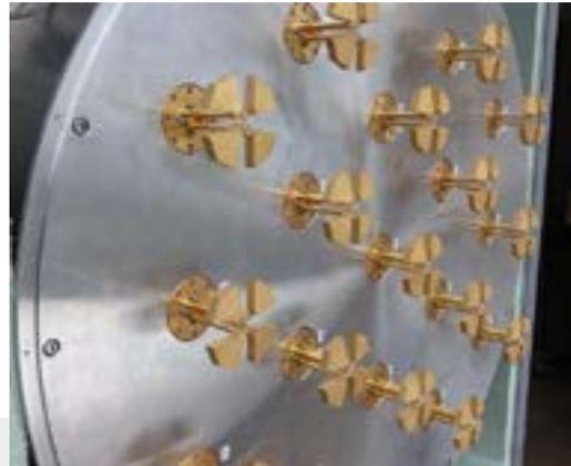
[The 19-element phased array feed developed by the NRAO CDL.](#)
