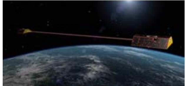
This illustration of the GRACE-FO mission shows two satellites orbiting Earth together. When the satellites' orbit takes them over a massive object, such as a mountain or aquifer, the object's gravitational pull will change the distance between the satellites. By tracking these variations, researchers will be able to study how the distribution of Earth's water changes over time. NASA/JPL-Caltech
