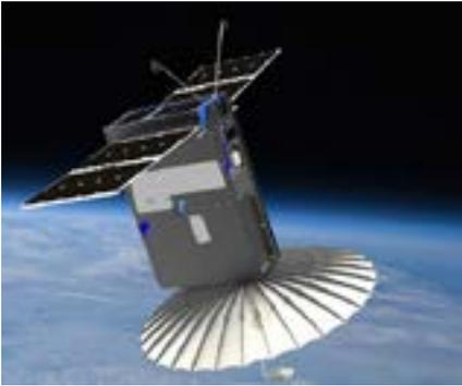
The RainCube 6U CubeSat with fully-deployed antenna.
