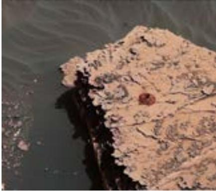
NASA's Curiosity Mars rover captured this shot of the 2-inch-deep (5 centimeters) hole it drilled in a target called "Duluth" on May 20, 2018. It was the first rock sample captured by the drill since October 2016. Credit: NASA/JPL-Caltech/MSSS
