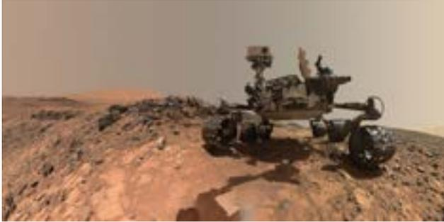
This self-portrait of the Mars Curiosity rover reveals a rock stuck to the left middle wheel. NASA Jet Propulsion Laboratory
