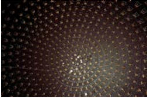
This interior view of the MiniBooNE detector tank shows the array of photodetectors used to pick up the light particles that are created when a neutrino interacts with a nucleus inside the tank. Credit: Fermilab / Reidar Hahn
