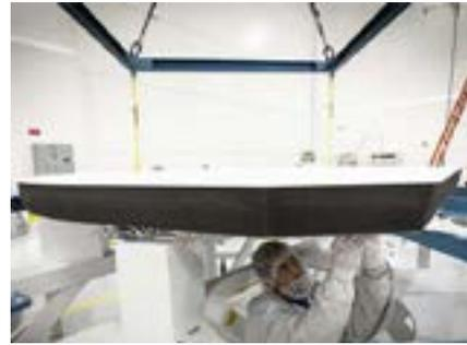
[The Thermal Protection System connects to the custom-welded truss on the Parker Solar Probe spacecraft at six points to minimize heat conduction.](#)
