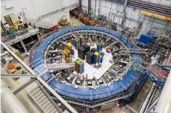
The Muon g-2 storage ring installed and ready to take data at Fermi National Accelerator Laboratory. Credit: Fermilab
