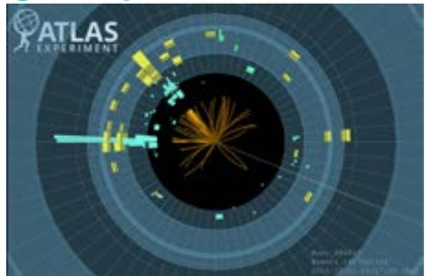
Event display for the  $H \rightarrow b\bar{b}$  decay analysis with the ATLAS detector. Credit: ATLAS Collaboration/CERN
