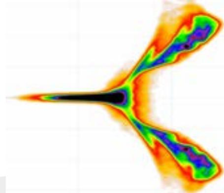
Simulation of groups of positrons being concentrated into a beam and accelerated. Credit: Aakash Sahai
