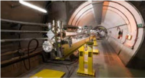
In a demonstration of a new particle accelerator technology, physicists with the AWAKE experiment (plasma cell, shown) accelerated electrons on the wakes of protons plowing through plasma.
