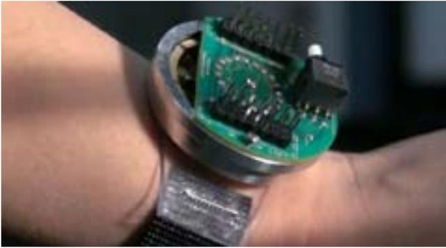
A piezoelectric energy harvester in a novel wristwatch-like device. Credit: Penn State
