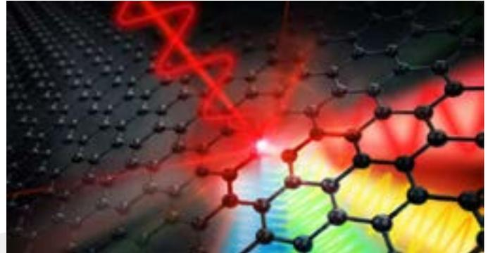
**SPECTRAL SPECTACLE** New experiments show that graphene is especially good at translating incoming signals of one frequency (illustrated in red) into signals of higher frequencies (yellow, green and blue).
