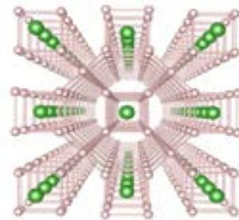
**HELLA HYDROGEN** The compound LaH10 is composed of 10 hydrogen atoms (pink) for each lanthanum atom (green). This hydrogen-rich material was predicted to exhibit superconductivity, evidence for which has now been found.
