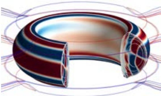
The color-shaded regions on the smooth doughnut-shaped surface of the KSTAR plasma, together with the external 3D field coils in blue and red used to generate the distortion. Credit: Jong-Kyu Park, Princeton Plasma Physics Laboratory.
