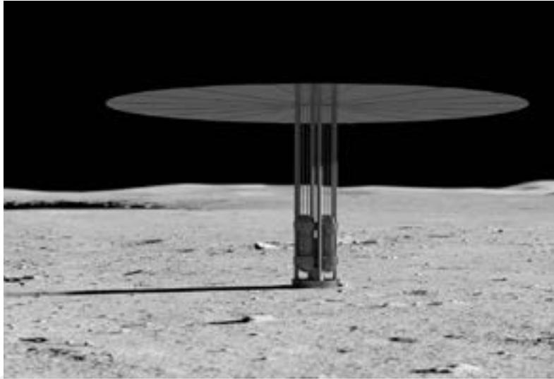
The Kilopower small nuclear reactor could be tested on the moon in the coming years. NASA
