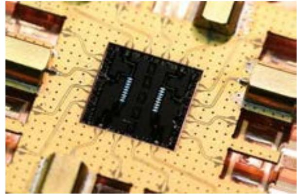
A superconducting metamaterial chip mounted into a microwave test package. The purplish-violet reflection in the center is an optical effect that can be seen by the naked eye, and is the result of the diffraction of light by the periodic patterning of the microwave metamaterial. Credit: Oskar Painter/Caltech
