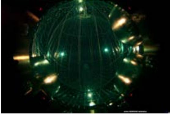
The Borexino instrument located deep beneath Italy's Apennine Mountains detects neutrinos as they interact with the electrons of an ultra-pure organic liquid scintillator at the center of a large sphere surrounded by 1,000 tons of water. Credit: Borexino
