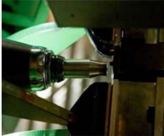
Close-up view of a friction stir weld tack tool used to manufacture external tanks of the space shuttle. Friction stir welding is different from traditional fusion welding in that the materials are not melted.
