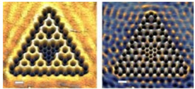
Electrons in bonding (left) and non-bonding (right) Sierpinski triangles; scale bar 2nm. Credit: Kempkes et al., *Nature Physics*, 2018
