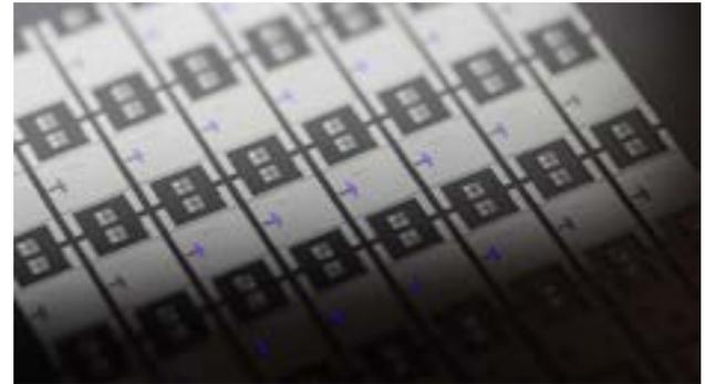
An array of the acoustic wave devices used in the experiment on quantum circuits. The bright purple part is the active part of the device. Credit: Kevin J. Satzinger
