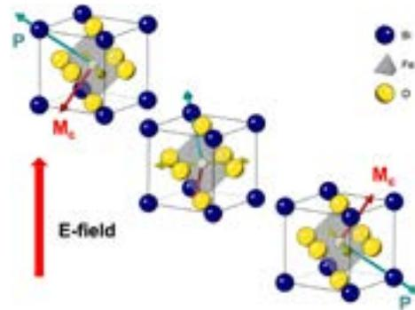
MESO devices, based on magneto-electric and spin-orbit materials, could someday replace the ubiquitous semiconductor transistor, today represented by CMOS. MESO uses up-and-down magnetic spin states in a multiferroic material to store binary information and conduct logic operations. Credit: Intel graphic
