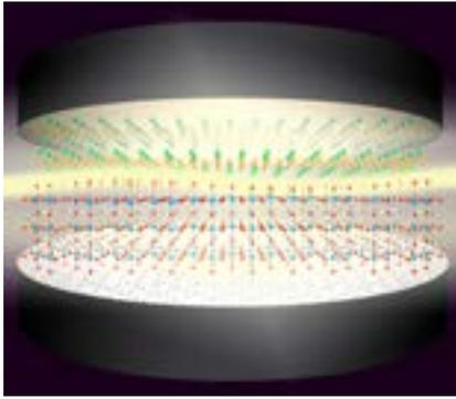
The vacuum fluctuations of light (yellow wave) are amplified in an optical cavity (upper and lower reflecting mirrors). Crystal lattice vibrations (red atoms) at a two-dimensional interface surf this strong light wave. The thus mixed light-vibrational waves couple particularly strongly to electrons in a two-dimensional atomically thin material (green and yellow atoms), changing its properties. Credit: J. M. Harms, MPSD
