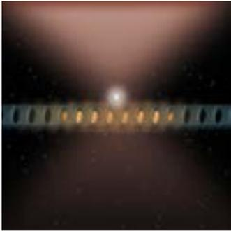
Researchers have used a light-guiding nanoscale device (blue structure) to measure and control position of a nanoparticle (white blur) in an optical trap (red light). This is possible because the light guided in the photonic crystal cavity is influenced by the motion of the particle. Credit: Lorenzo Magrini, University of Vienna
