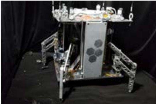
By using steam rather than fuel, the World Is Not Enough (WINE) spacecraft prototype can theoretically explore “forever,” as long as water and sufficiently low gravity is present. University of Central Florida
