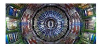
The Compact Muon Solenoid detector is a general-purpose detector at the Large Hadron Collider (LHC) in Switzerland, designed to observe any new physics phenomena that the LHC might reveal. Credit: CERN
