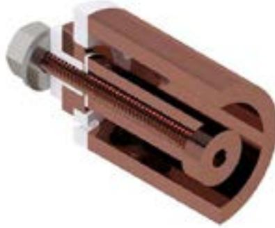
This rendering depicts a device that electromagnetically accelerates plasma to produce thrust - contrasting typical chemical thrusters. In order to create the propellant plasma, a low energy surface flashover (LESF) technique is employed at the beginning of the channel.
